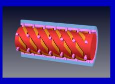
These mixers can be used in extrusion, compounding, direct-extrusion, foam extrusion, blow molding, and directinjection molding. The VIP mixer fits in a conventional smooth barrel and, therefore, can be used in standard extruders and injection molding machines. Installation of the intermeshing pin mixer does not require modification of the extruder barrel or a barrel extension. As a result, installation is simple and straightforward.
