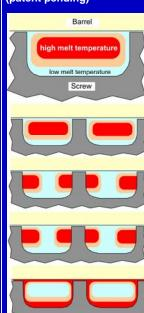
gion and vice versa. A new screw geometry has been developed which forces high temperature melt in the center region of the channel to the barrel surface. This new screw has been used in polystyrene foam extrusion to improve the cooling capacity of the secondary extruder. The HHT screw improved the cooling capacity by 25%-50% relative to the existing
