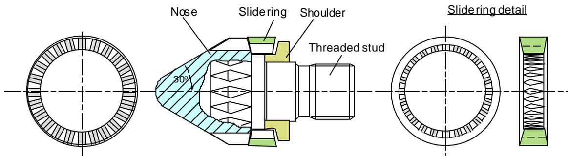
Figure 4, CRD non-return valve for injection molding screws (open position)
