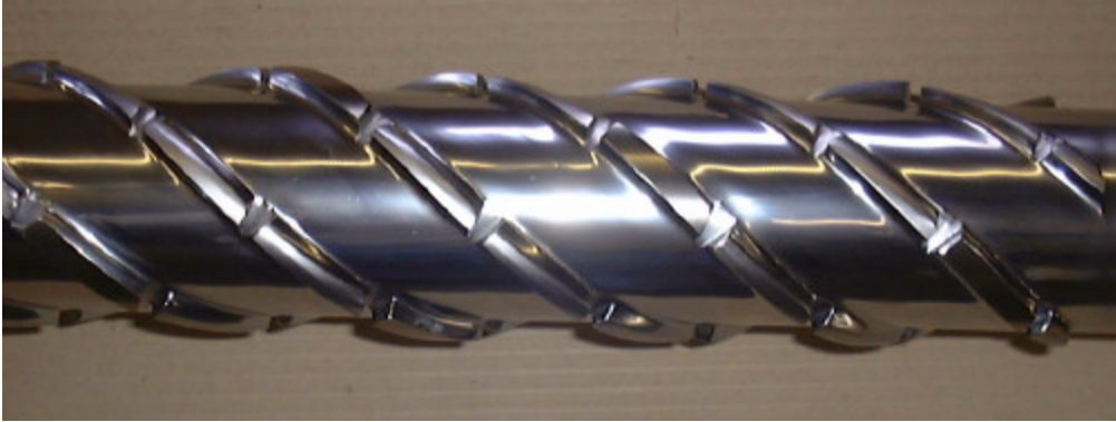
Figure 3, CRD 5 mixing section
