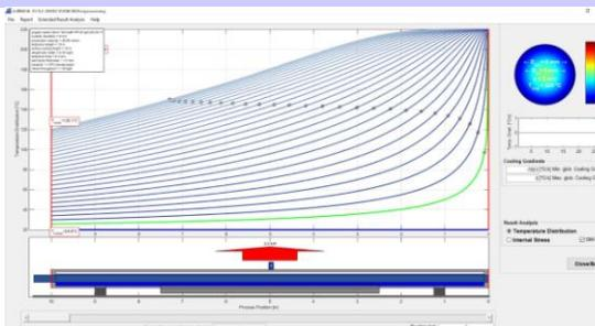
6-mm PP rod extruded at 43 kg/hr, 10 meter long cooling bath
