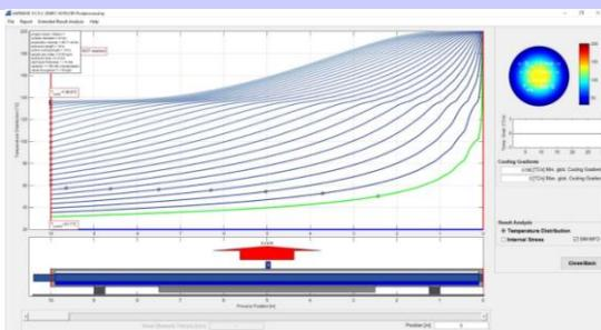
6-mm HDPE rod extruded at 43 kg/hr with 10 meter long cooling bath
