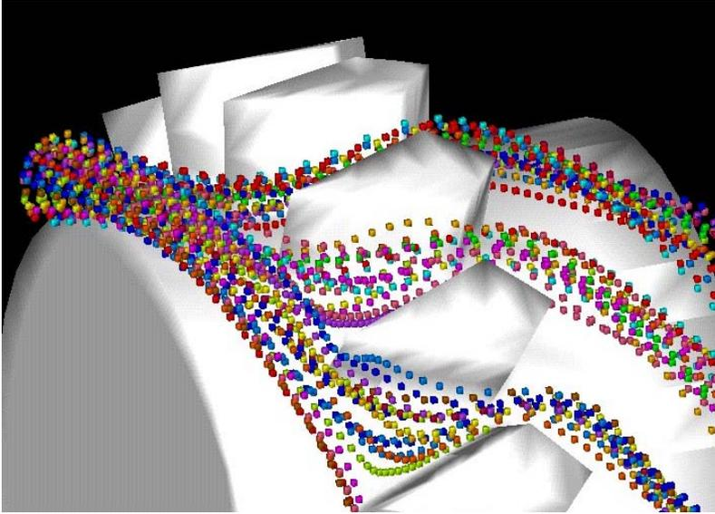
Figure 4, Particle tracking results in a mixing section with elongational mixing pins
